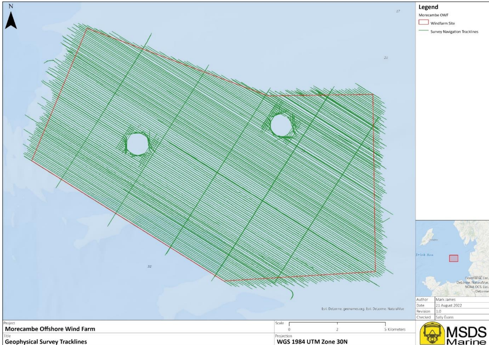
Figure 2: Geophysical survey tracklines (from MSDS, 2022)
